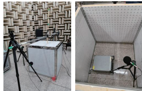
图9 分布式通风隔声罩性能测试的现场布设 Fig.9 Site layout for the performance test of the distributed ventilation and sound insulation shield
